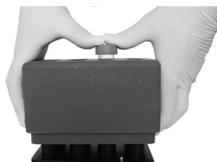
Fig 5 Push the cylindrical object down while pulling the external housing from the base to release the magnets. Pull the housing off the tube wells.
