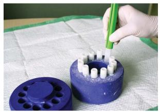
BioCision's CoolCell alcohol-free cell freezing containers ensure standardized controlled-rate -1°/min cell freezing in a -80°Cfreezer—without alcohol or any fluids.
